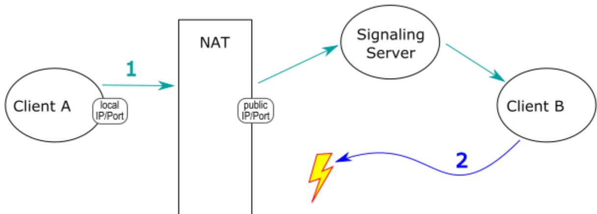
Fig. 2: Unsuccessful connection setup through a NAT router.
