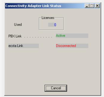
Install the ECSTA. At CAP Login use the option **OpenScape 4000** - **Native Mode CA4000**. In network conections use the host, where the CA4000 is installed and use the TSP port (default 1045) that you configured in the CA4000.
