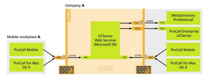
The following ports should be configured as part of a DMZ in principle, in order to make estos UCServer Web Services accessible from external networks (WAN), while protecting your Local Area Network (LAN) in contrast against external access.
