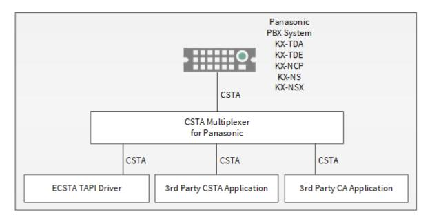
The CSTA Multiplexer connects to the PBX system. The CSTA Applications connect to the CSTA Multiplexer.
