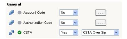
The CSTA Type must be set according to the connected device.
